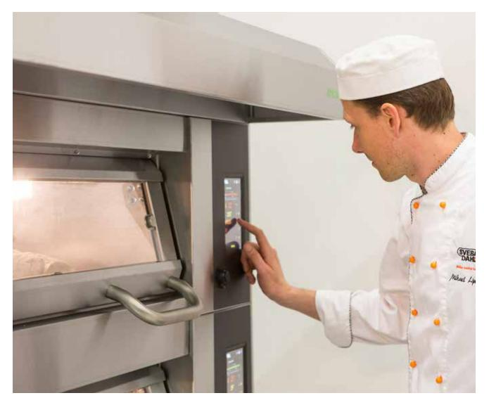
The D-Series has the option of selecting the eco+ concept. Our eco+ equipped ovens have been developed to meet the requirements for future energy savings. For this reason, we have looked at the oven as a whole. A product labelled with eco+ from Sveba-Dahlen has optimised software. In addition, the oven's walls, floor as well as the oven door are well insulated, to keep the heat in the oven, which gives a more comfortable climate in the room and a 35% saving in energy consumption.
