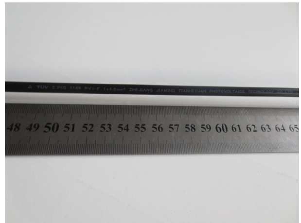
Cable(PV1-F 1 x 4.0mm 2 )
