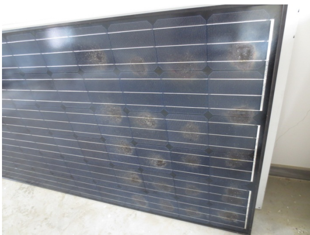
Sample 8#: After burning brand test
