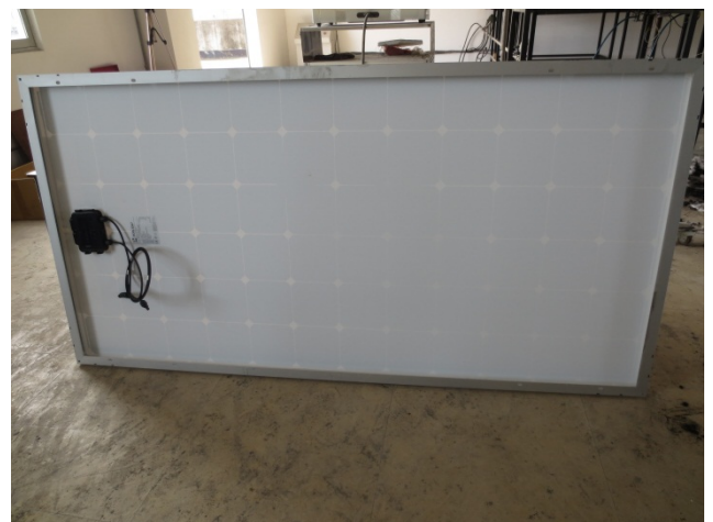
Sample 4#: After burning brand test
