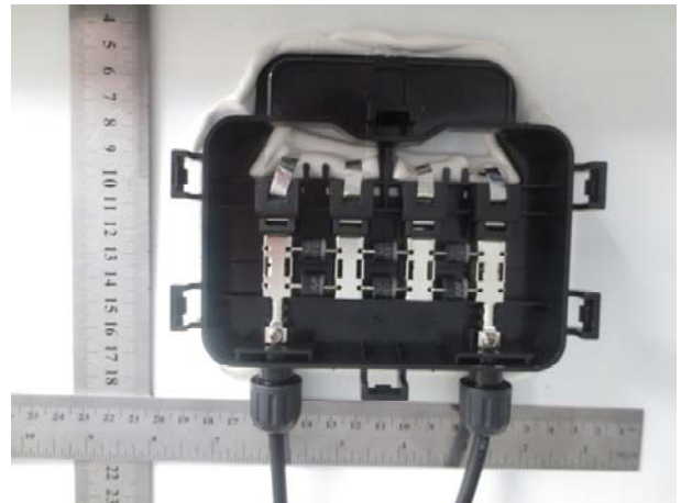
Junction box (opened)
