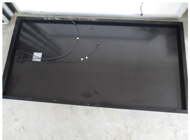
Sample 8#: After burning brand test
