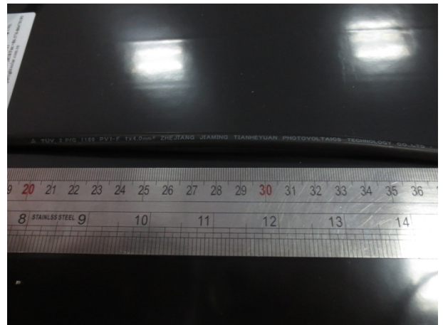
Cable(PV-F, 1 x 4.0mm 2 )
