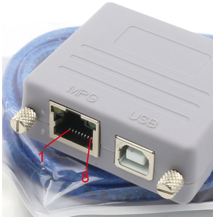
Figure2-4. Pins Number of MPG
