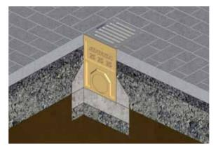
Install paving. The layer should end 2 to 5 mm higher than the cover grating.
