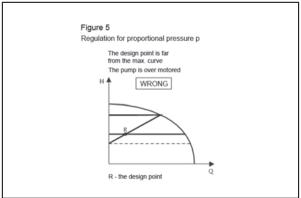
While using regulated pumps you can benefit from the operational field of a particular pump, which ranges from the minimal to the maximal Q-H curves. That is why such a regulation type is called stepless thermal regulation. The R design point should be located as close as possible to the functional max. Q-H curve.
