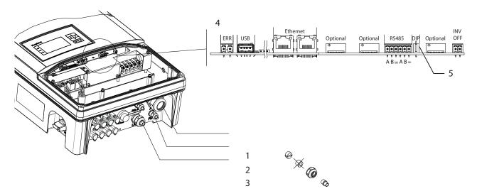
Figure 22: Connection area: Connection and assignment of the interfaces
