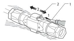
Figure 32: Disconnect connector
