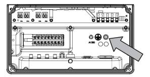
Figure 21: Grounding point in the connection area
