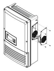
Figure 29: Removing the cover and fan from the housing
