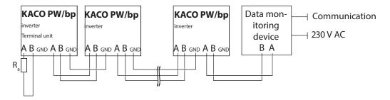
Figure 23: RS485 interface wiring diagram
