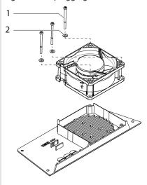
Figure 31: Mounting the fan
