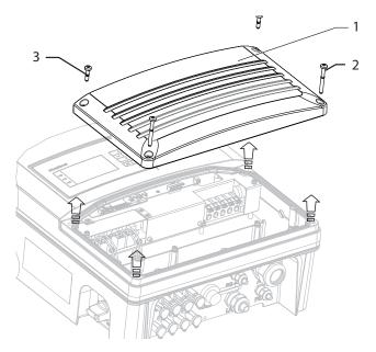
Figure 12: Connection area: Open connection cover
