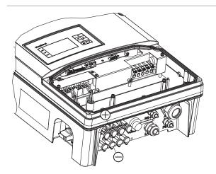
Figure 18: Connections for DC positive and DC negative
