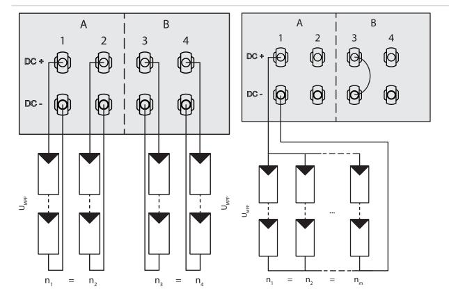
Figure 19: Recommended standard connection
