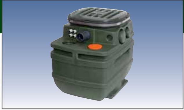
Automatic collection and lifting stations, used for collecting and pumping civil and industrial waste water in sewers. Comprises a high density 280 litre polythene tank with removable cover complete with a watertight and gastight seal. Complete with lifting device (DSD2) for making pump maintenance easier. Fitted for one automatic electric pump (**FEKA 600 M-A - FEKA VS 550 M/A - FEKA VS 750 M/A - FEKA VX 550 M/A - FEKA VX 750 M/A**) to be ordered separately.
