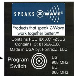
**Inclusion** in (adding to) a network: 1) Set up the inclusion mode at the controller; 2) Briefly press the button once and the controller will indicate the unit has been included in the network. Also, the LED will blink when the inclusion completes. *Inclusion and exclusion are always done at normal transmit power mode.*
