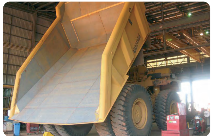
Mining vehicle. Matrox-lined truck bed for ore transport in Australia
