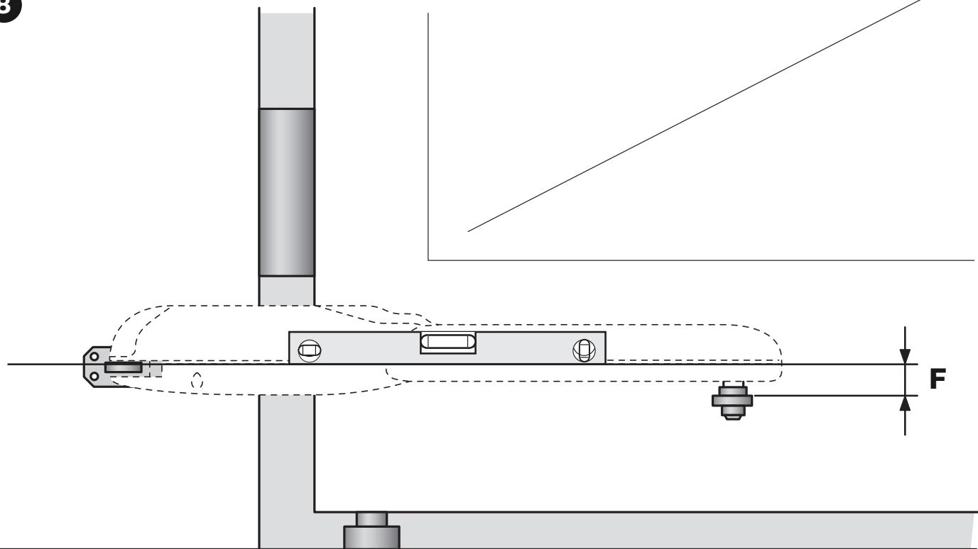
**WG4025 - WG4000 - WG4000/V1:  $F = 30 \text{ MM}$**
