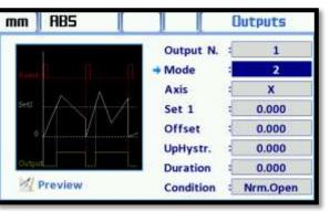
If the duration is not entered in, the output remains active, if the duration is entered, the output is remains active during the entered time and then switches to passive position. The output remains active unless it comes buton ( reset the axis) or reset the signal. Optionally, histeric and offset values can be entered.
