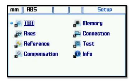
System Setup menu options include directional move with arrow keys when in the desired option, and sub-menu with "ENT" button can be entered. Shortcuts to navigate to the desired option available and It can use the numeric buttons for this operation (to compensation menu it used "3" button).
