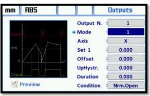
When the axis value falls below from set value the output is passive without depending on the duration value is entered. Optionally, histeric and offset values can be entered.
