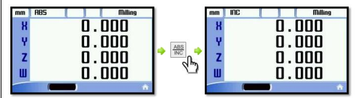
The mode of operation used in the upper left corner of the screen next to the measuring system is indicated.
