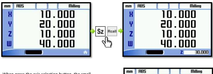
When press the axis selection button, the small window at bottom right opens. "Rcall" button pressure the previous value appears in this window. "ENT" button is pressed, this value is transferred to the axis. In case of cancellation of transfer value press "Esc" button instead of "ENT".
