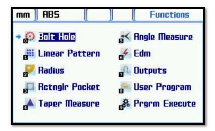
Among the options at the functions of menu can be moving with the arrow keys and when the desired options, it can be entered in submenu with "ENT" button. Shortcuts are available to move the desired option with numeric buttons. ("2" button is used to "Radius" menu).
