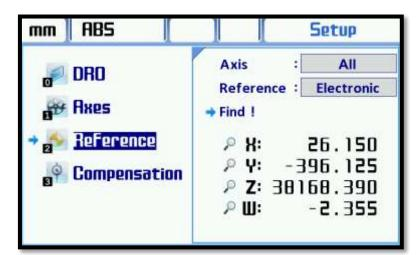
Encoder is moved until to recieve the reference signal. the check icon will be appeared next to the Axis which get reference signal and axis will be reset.
