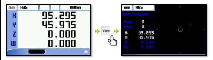
The "View" button is pressed, the screen, the X and Y axes of the coordinate system will be located. The current position is on the left with white text to be specified and will be displayed on the yellow pointer with coordinate system. The display mode again to exit the "View" button or the "Esc" button must be pressed.
