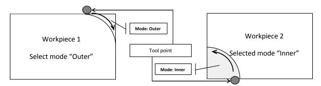
Enter radius of the circular area on the "Radius" line. Enter tool diameter of workpiece on the "Tool Dia" line. The angle of starting point process on "Angle 1" line, the angle of end process on "Angle 1" line should be entered. The maximum value of between the two points to be drilled is entered on the "Max Cut" line.
