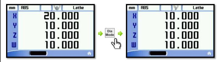
In the example above, the diameter mode which is open was closed. To turn it on again, "Dia Mode" button is used. When diameter mode turn on, the icon of diameter is located next to bench type the upper side on the LCD. When the diameter mode turn off. The icon changes and becomes an icon that measures the radius.
