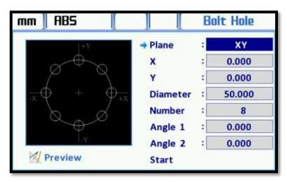
8-line display comes on the screen. The plane which the process to apply is determined with direction arrows on the "Plane" line and selected with "ENT" button.
