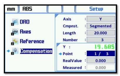
Second line on the "Point" line is displayed count of correction point. Scroll to the required correction point. It is shown as a "A / B", A; count of point and B; total number of correction point. In the above example; it is understood that there are 3 correction point and at the 1. Point.
