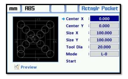
An screen is displayed 8 lines. The distance of starting point(center point) to X axis is entered on the "Center X" line. The distance of starting point(center point) to Y axis is entered on the "Center Y" line. The size of discharged pool on the X-axis length on the "Size X" line, The size of discharged pool on the Y-axis length on the "Size Y" line is entered. The diameter of the tool used to workpiece is entered on the "Tool Dia".
