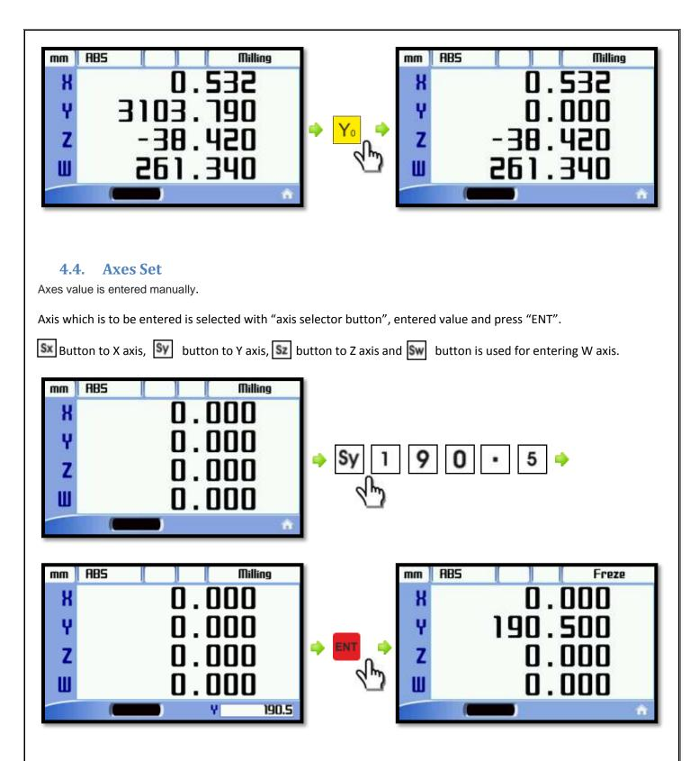
Select the axis to be entered by pressing a small window appears at the bottom right of the screen. Value will appear on the display until press "ENT". "ENT" button is pressed, the value is transferred to the axis.
