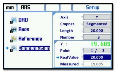
when the correction point is saved, 4. line measured value is displayed. the next point is displayed on the "Point" line and the same process is repeated for this point.
