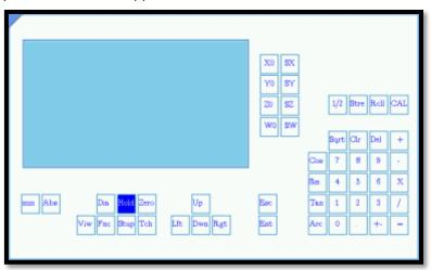
Keyboard test screen when pressing the button, the display changes to blue. All the buttons are pressed and the keyboard test in the same screen, the button that is marked to be seen.
