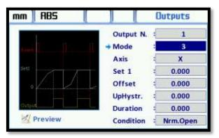
If the duration is entered, the output is remains active during the entered time and axis value remains in the locked position. End of the duration, the output becomes passive and Axis value is reset. Optionally, histeric and offset values can be entered. Hysteresis lower rate is not used this mode.
