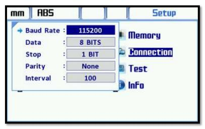
Value of Baud Rate, Parity, stop bits, and periods can be modified in this menu.
