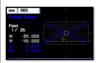
When the function startup the simulation screen will be open like a the side. The current position is shown with a yellow marker.
