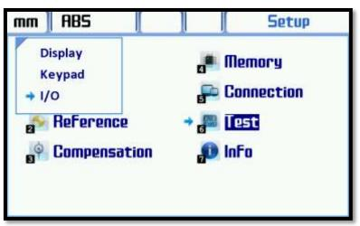
When press "0" EDM relay, press "1" exit-1, press "2" exit-2, press "3" exit-3, press "4" exit-4, press "5" exit-5, press "6" exit-6 will be active. If the same button is pressed again the output will be passive.
