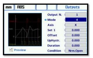
When the output is active it can be passive position again with button (reset axis) or reference sensor of sensor. Optionally, histeric and offset values can be entered.
