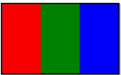
After the Test the LCD screen respectively would be white, red, green, and blue. Thus, in the case of any problems such as dead pixel problem is seen in a clear manner.
