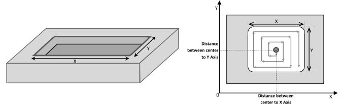
To enter the the Rectangular Pocket, press "3" button while on the function screen or to reach the "Rctnglr Pocket" with arrow keys then press "ENT" button.
