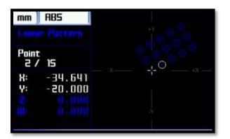
The first point can be processed and when press "ENT" or down arrow button the second point is displayed on the simulation screen as a white.
