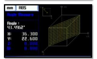
When the function startup the simulation screen will be open like a the side. The measuring axis should be chosen with up and down arrow buttons. The selected axis will be displayed as a white in the list on the left.
