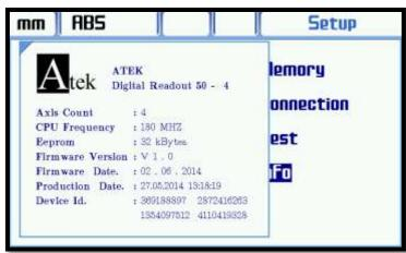
In the window that opens, the number of CPU frequency axis, Eeprom, version, software date, production date and device ID is located.
