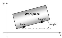
To enter the Angle Measure Function, press "5" button while on the function screen or to reach the "Angle Measure" with arrow keys then press "ENT" button.
