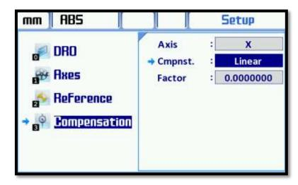
The bottom line will be appeared on the screen. To entered that calculated correction factor on the this line and save with "ENT" button. After the finishing of this function set, log out with "Esc" button
