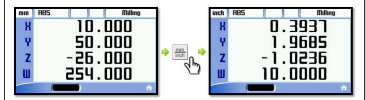
Used measuring system is noted in the upper-left corner of the screen.Measurement system is changed, the values on the screen are converted according to the new system..
