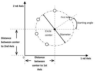
To enter the divisor menu, press "0" button while on the function screen or to reach the divisor with arrow keys. then press "ENT" button.
