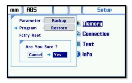
In order to erase all programs, the selected "Erase" on the program line and press "ENT" botton. A query window will open. "Are you sure?" query "Yes" is selected. The screen that opens "Erasing" is displayed. All programs have been erased.
