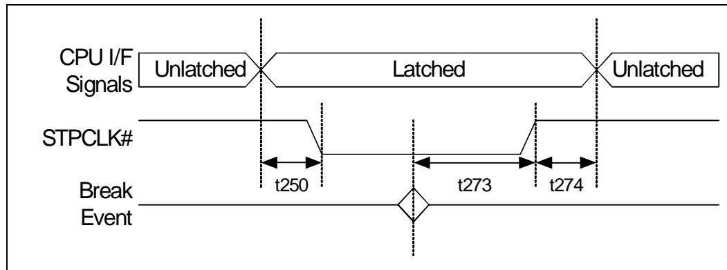
Figure 8-20. C0 to C3 to C0 Timings (Mobile Only)
