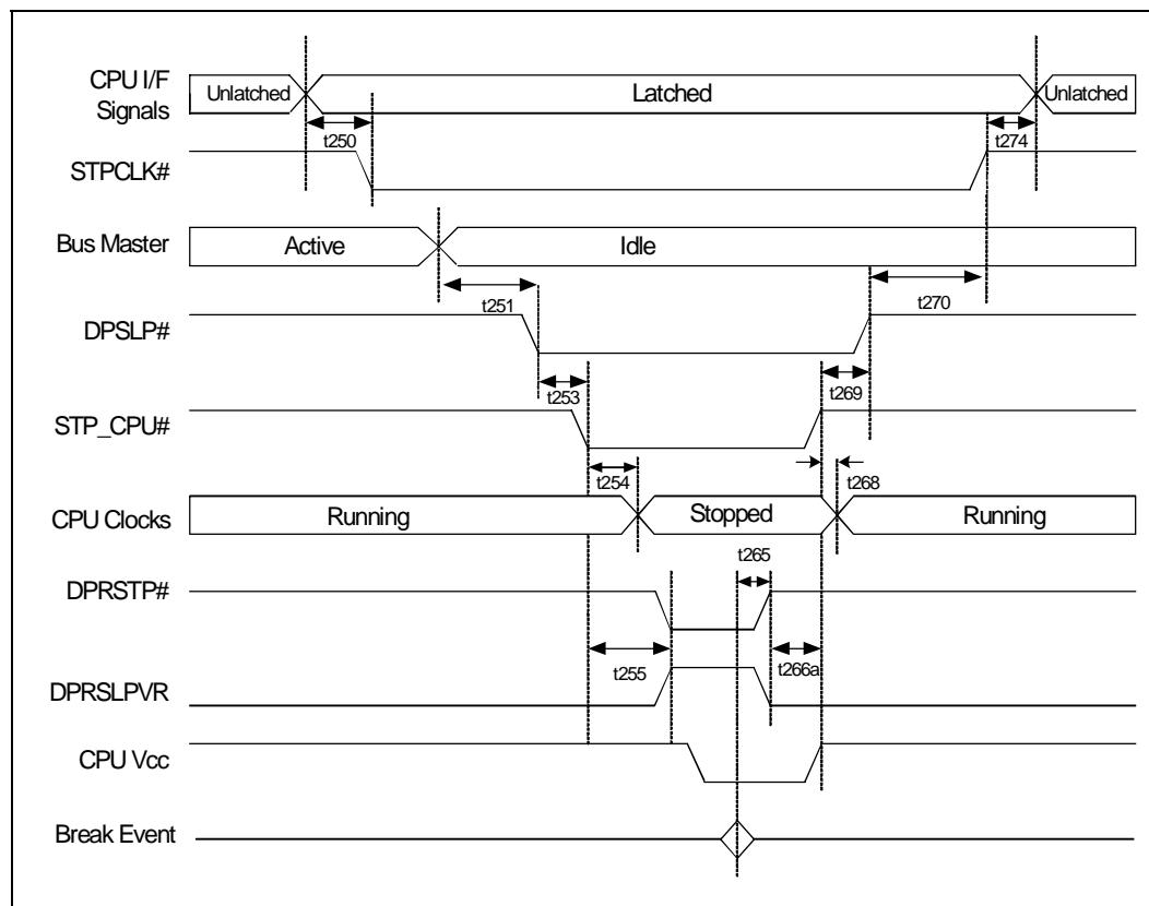
**Figure 8-22. C0 to C5/C6 to C0 Timings (Mobile Only)**
