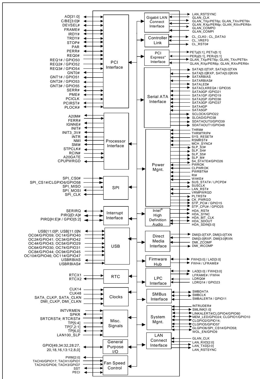
Figure 2-2. Intel® ICH9 Interface Signals Block Diagram (Mobile)
