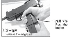
注意:請勿使彈匣直接掉落地面,以防止 變形或損壞。 JTION: Magazine falling directly on the ground could cause deform or damage on it.
