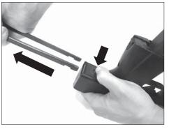
移除槍身前端的插銷和軸 Remove frame bolt and frame pin.
