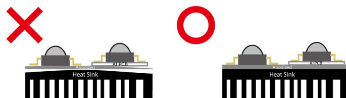
< Figure 31. Edixeon® series assemble with heatsink >
