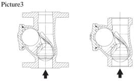
Piping with horizontal or inclined flow (upstream flow): install the valve as shown in figure 4.
