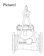
Piping with vertical upstream flow: install the valve as shown in figure 3.
