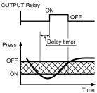
\*In case pressure decrease than the ON pressure during working of Delay timer, timer is reset, and dose not turn on.
