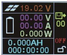
Power display interface, showing currently measured solar panel voltage 19.02V.
