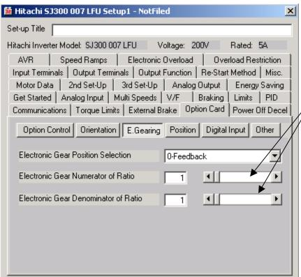
After initial electronic gearing tests are performed, the gearing ratio can be changed by these parameters (P20 & P21).
