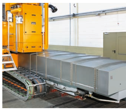
■ Telescopic cover for lathes
