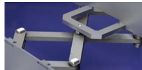
5 Synchronising device (harnesses) for fast-running telescopic covers
