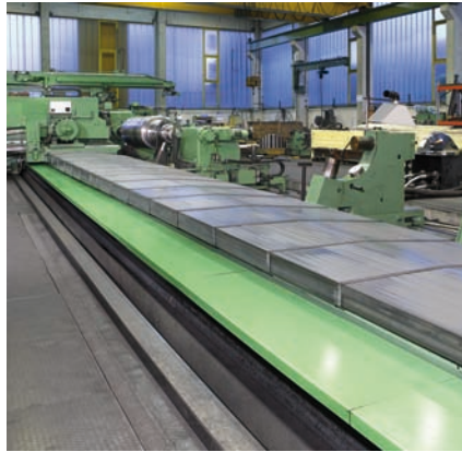
■ Telescopic cover for wheel grinders
