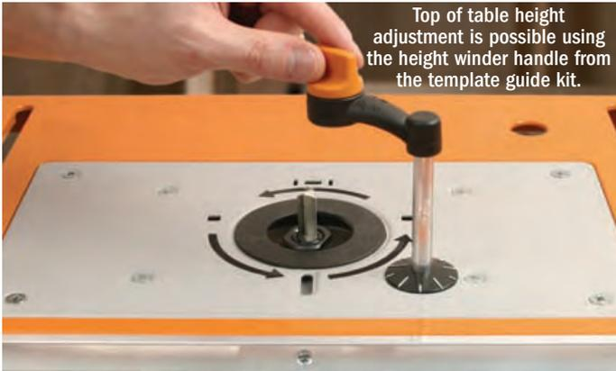
Top of table height adjustment is possible using the height winder handle from the template guide kit.
