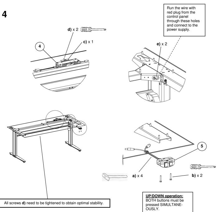
To ensure correct up and down operation of the desk frame it has to be fitted with a tabletop or applied a similar weight. Without a tabletop fitted, the desk frame may not operate in the downward direction.
