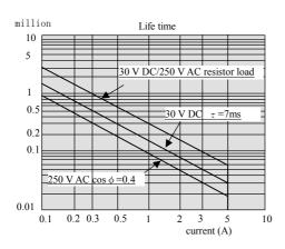
Since the lifetime of relay contact is in inverse proportion to squared current, be aware that interrupting rush current or directly driving the condenser load will drastically reduce the life of the relay.
