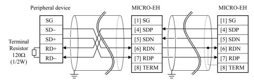
Use a terminal resistor if necessary
