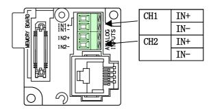
Figure. 9.3 Analog input terminals on option board
