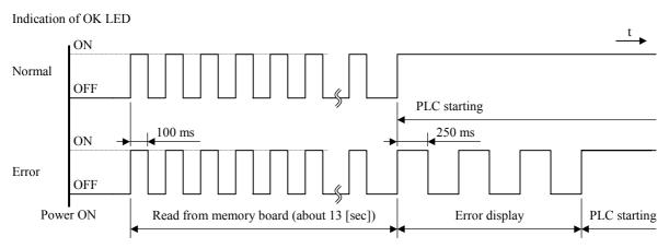
Figure 9.1 OK LED indication (In case of the memory board mount)
