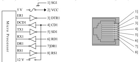
Figure 5.2 Circuit diagram and pin numbers for port
