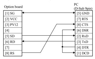
Standard RS-232C communication cable for the existing port on basic unit can be used with this option port too.
