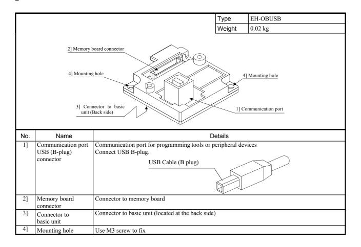
Since this board is a converter from RS-232C to USB, the USB port of PC must be regarded as RS-232C port. For this reason, COM port driver is necessary for your PC. Please download the driver from following URL and install so that USB port works as serial port.
