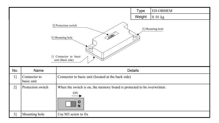
The function of the memory board is to save user program and data in special internal outputs. It is also possible to read out to PLC, which enables users to copy program (incl. data in special internal outputs) without programming software or peripheral devices.
