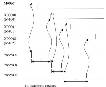
In the program example described previously, the external I/O (X, Y) are used as switch signals of a process; thus, the time for performing I/O refresh (i.e., at least one scan period) is required for each process.
