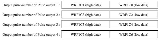
Figure 4.11 Special Internal output for an Pulse output setup
