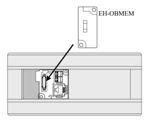
(2) Fix by attached a tapping screw.
