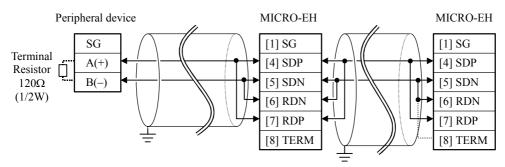
Use a terminal resistor if necessary
