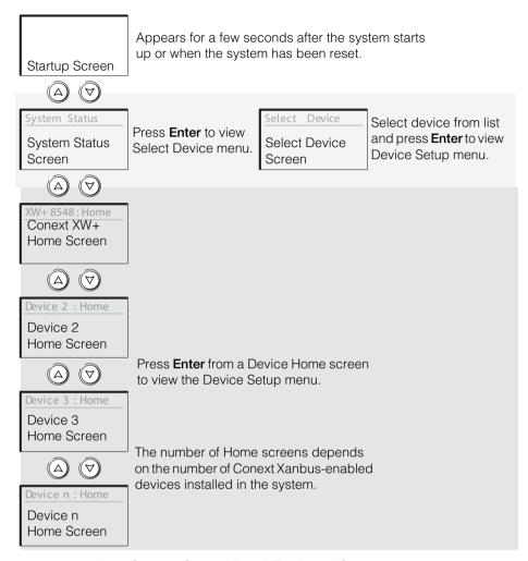
Figure 2-4 Xanbus System Control Panel Top Level Screens
