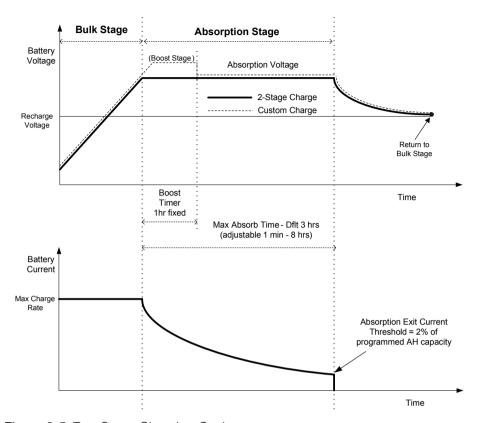
Figure 3-5 Two-Stage Charging Cycle
