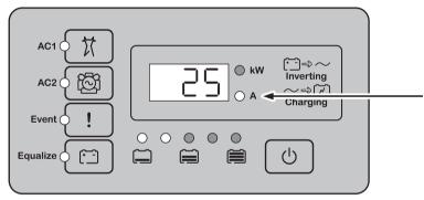
Figure 2-3 Inverter Information Panel When Charging Battery
