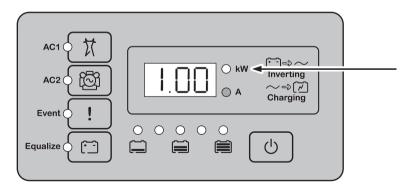
Figure 2-2 Inverter Information Panel When Inverting
