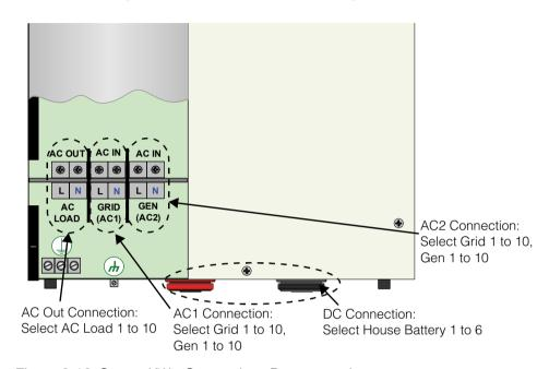
Figure 3-12 Conext XW+ Connections Representation
