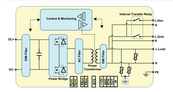
Figure A-6 Conext XW+ Block Diagram
