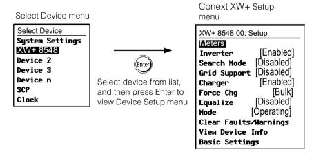
Figure 2-5 Selecting a Device Setup Menu
