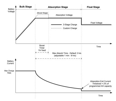
Figure 3-4 Three-Stage Battery Charging Cycle
