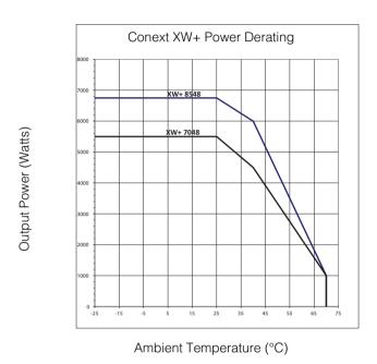
Figure A-2 Output Power Versus Ambient Temperature
