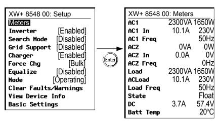
Figure 2-8 Viewing the Meters Screen
