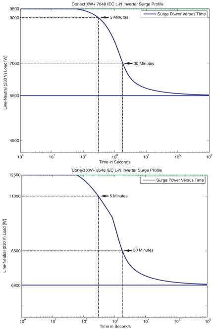
Figure A-1 Conext XW+ AC Overload Capability
