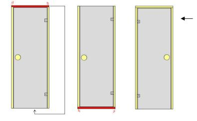
\* If it is necessary to change hanging, move the top rail to the other end. Put the door on the floor, unscrew the upper horizontal detail's four screws, put the horizontal on the opposite side of the door and screw it back with the same four screws. Now it's ready.
