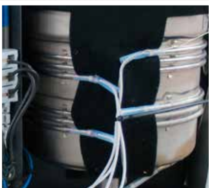
Heating elements are welded like a coil around the water tank and have no direct contact to water.
