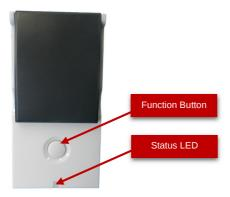
The device is able to switch electric loads up to 3500 W and can be switched wirelessly or using the local button.
