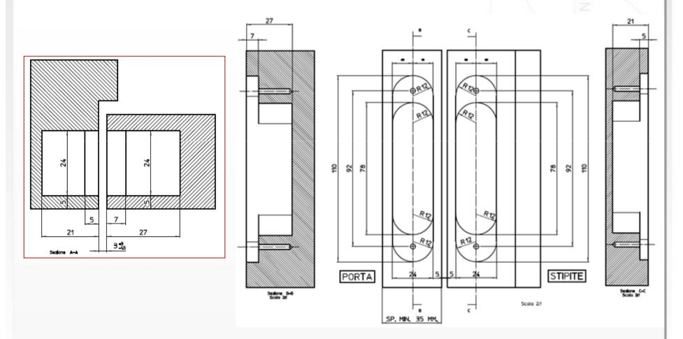
Load capacity: 40Kg with n.2 hinges - 52Kg with n.3 hinges
