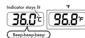
The [°C (°F)] indicator symbol will stop blinking and stay on when the reading is ready.
