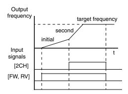
In the graph shown above, the [2CH] signal becomes active during acceleration. This causes the inverter to switch from using acceleration 1 (F002) to acceleration 2 (A092).
