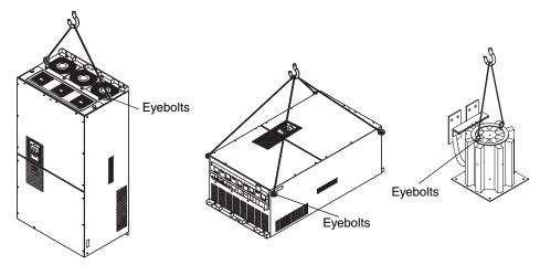
Upright inverter lifting: Use eyebolts at top of inverter
