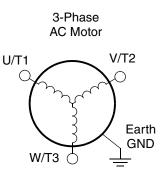
Notice the three connections to the motor do not include one marked "Neutral" or "Return." The motor represents a balanced "Y" impedance to the inverter, so there is no need for a separate return. In other words, each of the three "Hot" connections serves also as a return for the other connections, because of their phase relationship.
