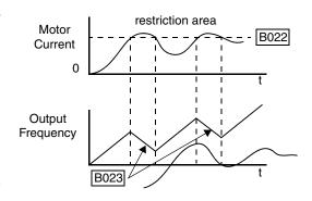
controlled deceleration, the inverter monitors both output current and DC bus voltage. The inverter will increase output frequency to try to avoid a trip due to over-current or over-voltage (due to regeneration).
