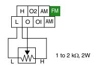
**Voltage Input** – The 0–10V voltage input circuit uses terminals [L] and [O]. Attach the signal cable's shield wire to terminal [L] on the inverter only. DO NOT ground the shield at its other end. Maintain the voltage within specifications (do not apply negative voltage). Normally a full-span input level (10V) will give the maximum motor frequency. You can use parameter A014 to select a lower voltage for full output frequency (such as using a 5V input signal).
