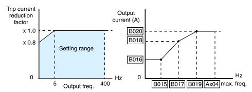
Suppose the electronic thermal setting (B012) is set to 44 Amperes. The left graph below shows the effect of the free setting torque characteristic curve. For example, at (B017) Hz, the output current level to cause overheating in a fixed time period is reduced by a factor of (B018). The right graph below shows the reduced trip current levels in those conditions for given trip times.
