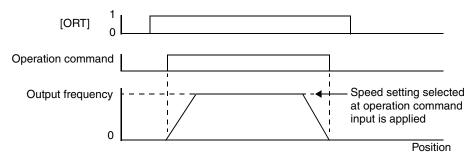
Teaching operation can be performed when power is input to the power supply terminals [R0] and [T0] of the inverter control circuit. The current position counter also operates when an external device moves the work piece. Therefore, the teaching operation can also be performed when the inverter does not operate (move) the machine.
