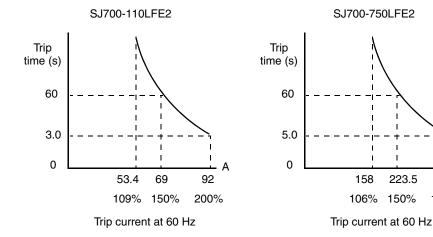
Example 3, setting for SJ700-3150LFE2 (185 to 400kW) - The rated motor current is 600A. The setting range is (0.2\*64) to rated current, or 120A to 600A. For a setting of B012=600A (current at 100% rated current), the curve is shown to the right.
