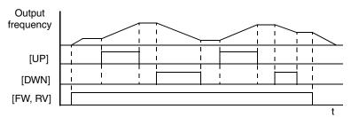
It is possible for the inverter to retain the frequency set from the [UP] and [DWN] terminals through a power loss. Parameter C101 enables/disables the memory. If disabled, the inverter retains the last frequency before an UP/DWN adjustment. Use the [UDC] terminal to clear the memory and return to the original set output frequency.
