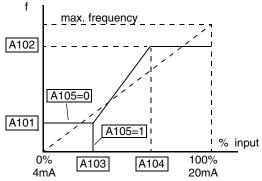
than the A104 ending value, the inverter outputs the ending frequency specified by A102.
