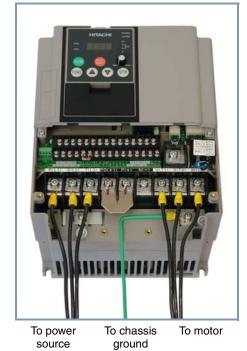
Use the same wire gauge on the motor and chassis ground wiring as you used on the power input wiring in the previous step. After completing the wiring:
