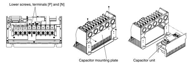
To install the new capacitor unit:
