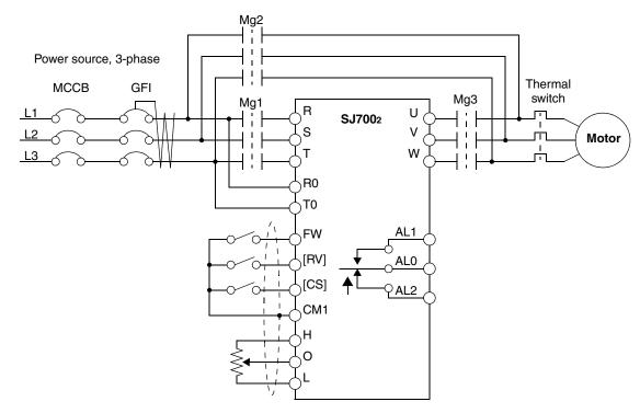
Switching to inverter control occurs after the motor is running at full speed. First, Mg2 relay contacts open. Then about 0.5 to 1 seconds later, relay Mg3 contacts close, connecting the inverter to the motor. The following timing diagram shows the event sequence:
