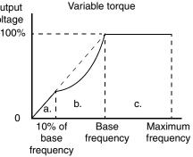
The graph above (right) shows the general characteristic for variable torque. The curve may be best described in three sections, as follows:
