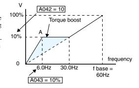
addition to the standard straight V/f line (constant torque curve).
