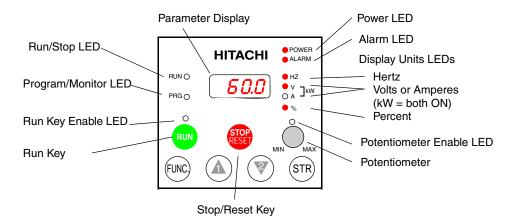
The display is used in programming the inverter's parameters, as well as monitoring specific parameter values during operation. Many functions are applicable only during the initial installation, while others are more useful for maintenance or monitoring.
