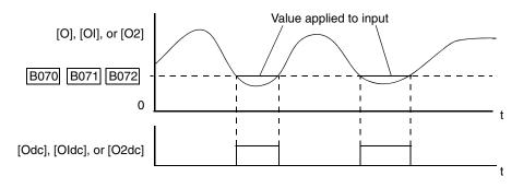
The inverter can also detect when an analog input value is within a range (or *window*) of values. See <u>"Window Comparator Signals" on page 4–62</u>.
