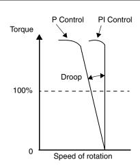
The proportional gain Kpp value determines the droop. Set the desired value using parameter
