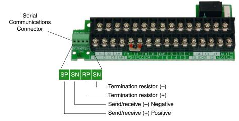
Each device requires just two connections in parallel for data transmission and reception. Additionally, the device at each physical end of the wiring requires a termination resistor. The SJ7002 has built-in termination resistors that become part of the circuit when you add a jumper as shown. The termination resistor helps to suppress electrical reflections.
