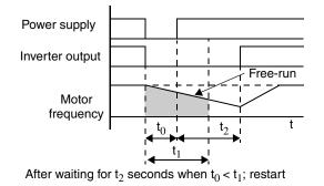
Example 2: Power failure longer than limits; trip
