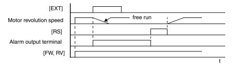
If the USP (Unattended Start Protection) feature is in use, the inverter will not automatically restart after cancelling the EXT trip event. In that case, it must receive either another Run command (OFF-to-ON transition), a keypad Reset command, or an [RS] intelligent terminal input signal.
