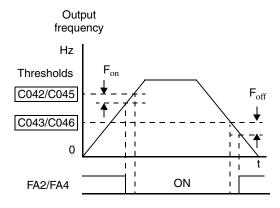
Frequency Arrival outputs [FA3] and [FA5] use the same threshold parameters as [FA2] and [FA4] above, but operate in a slightly different way. Refer to the diagram below. After the frequency arrives at the first threshold during acceleration and turns ON [FA3] or [FA5], they turn OFF again as the output frequency accelerates further. The second thresholds work similarly during deceleration. In this way, we have separate ON/OFF pulses for acceleration and deceleration.
