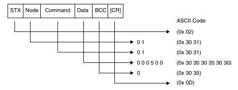
The block check code is computed by using the ASCII codes (shown above) and applying eXclusive OR (XOR) operations. Beginning with the first pair of bytes, the result of their XOR result is then used in an XOR operation with the third byte, and so on. For this example, the BCC calculation is shown below.
