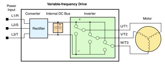
The simplified drawing of the inverter shows three double-throw switches. In Hitachi inverters, the switches are actually IGBTs (isolated gate bipolar transistors). Using a commutation algorithm, the microprocessor in the drive switches the IGBTs ON and OFF at a very high speed to create the desired output waveforms. The inductance of the motor windings helps smooth out the pulses.
