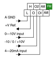
the inverter output frequency. The [AT] terminal function is covered in "Analog Input Current/Voltage Select" on page 4–24. Remember that you must also set A001 = 01 to select analog input as the frequency source.
