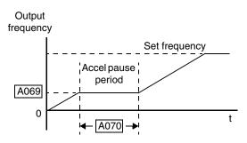
direction while the inverter is in a Stop mode. Initiating a normal acceleration in such a situation may result in over-current trips. This function can be used to keep the inverter output frequency and voltage at low levels long enough to bring the load to a stop, and commence turning in the desired direction before the acceleration ramp resumes. See also "DC Braking Settings" on page 3–18.
