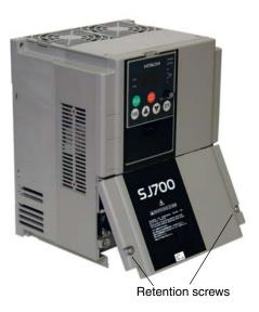
Notice the large power terminals at the bottom of the wiring area. The rubber grommets below the power terminals are for wire entry/exit to the power source and motor. Never operate the inverter with the front panel removed.
