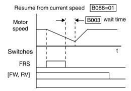
In the diagram above, [FRS] signal is active high. If you want the [FRS] terminal to be active low (normally closed logic), change the setting (C011 to C018) that corresponds to the input [1] to [8] that is assigned the [FRS] function (C001 to C008).
