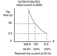
Constant Torque Characteristic – Selecting the constant torque characteristic for the example motor gives the curves below. At 2.5 Hz, the output current is reduced by a factor of 0.9 for given trip times.
