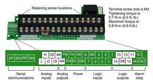
Specifications for the logic connection terminals are in the following table:
