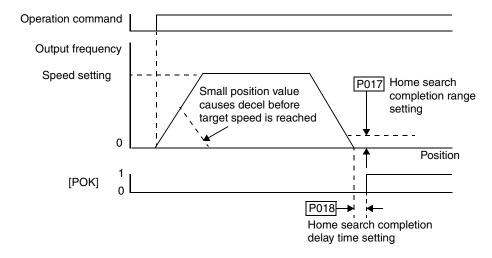
If zero return operation as described below is not performed, the motor position detected at powerup is assumed to be at the origin (position data = 0). When the operation commend is turned ON with zero specified as the position setting, positioning is completed without running the motor.
