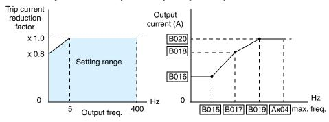
Suppose the electronic thermal setting (B012) is set to 44 Amperes. The graph below shows the effect of the free setting torque characteristic curve. For example, at (B017) Hz, the output current level to cause overheating in a fixed time period is reduced to (B018) A. Points (x), (y), and (z) show the adjusted trip current levels in those conditions for given trip times.
