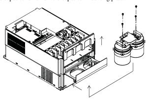
To install the new capacitor unit:
