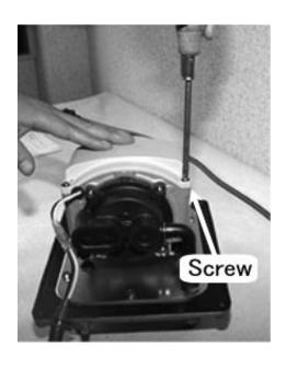
t) Put the shock absorber back into place.
