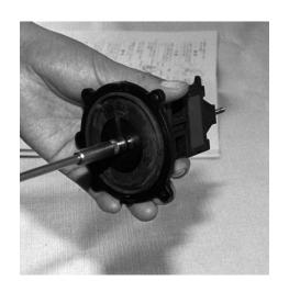
c) Assemble new magnet and diaphragm with nut or bolt.
