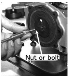
Undo the nut or bolt and remove the diaphragm (Nut: SLL series & EL-60, 80-15 & 120W - Bolt: EL-80-17, 100, 150 & 200).
