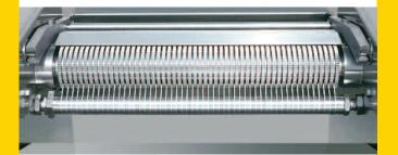
The automatic NOCK CBF machine models and the open top NOCK CF fish skinning machines are equipped with a **transport roller with grooves** (tooth roller). A **scraper comb** cuts in the grooves of the tooth roller and keeps it clean during operation.
