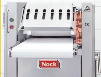
All machine parts which could obstruct the flow of the product, e.g. the mountings and handles of the blade holder, the mountings of the pressure device and of the conveyor belts, are located outside the tunnel-like safety cover.
