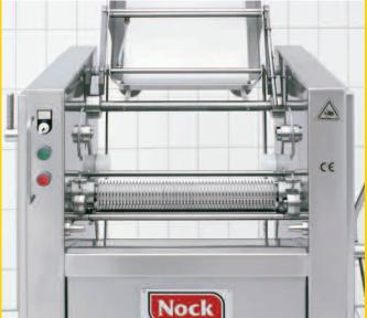
Quick and easy to clean: NOCK fish skinning machine after removing conveyor belts, pressure roller and blade holder
