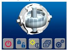
4) When the GYRO is turned off the flywheel is still spinning. When the flywheel has come to a complete stop <u>O RPM</u> will appear on the screen indicating that the flywheel has stopped. It can take up to 4.5+ hours for the flywheel to stop spinning.
