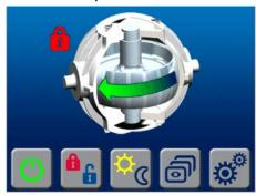
3) Press GYRO ON/OFF button. The ON/OFF symbol will turn RED
