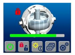
6) When the GYRO reaches its maximum operating speed where maximum stabilization is available, the PROGRESS BAR will disappear and the GYRO is available for maximum stabilization.
