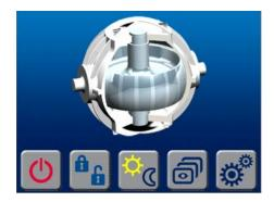
To turn the GYRO ON depress the POWER ON/OFF FAULT RESET button, the button will turn GREEN, the flywheel will spin (or arrow appear), and a RED PROGRESS BAR will appear. The PROGRESS BAR indicates how soon the gyro will be available for stabilization. When the Gyro is initialized and when the GYRO is up to minimum operating speed the PROGRESS BAR will turn from RED to GREEN. At this point, the GYRO is available for stabilization.
