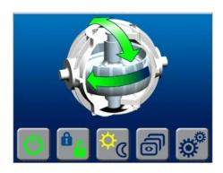
If it is necessary to shutoff power to the flywheel motor and slow the flywheel for any reason, press GYRO ON/OFF button; the button will turn RED and the LOCK/UNLOCK button will turn RED indicating the command has been accepted. It takes approximately 4.5+ hours for the speed to drop to zero rpm.
