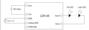
During analog dimming operation, Io will change with DC input voltage
