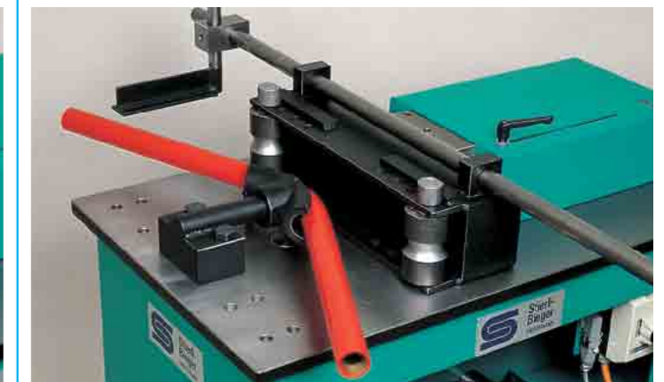
132 Gasrohrbiegen Bending of pipes
