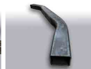
80 Grosse eckige Rohre biegen Bending of huge pipes
