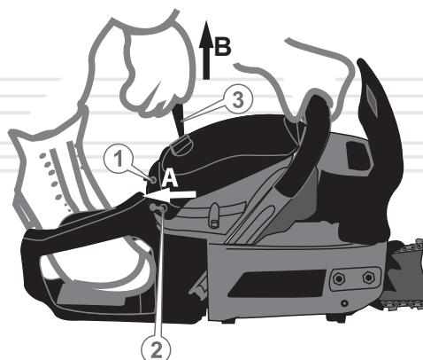
7. Pump the fuel to the carburetor, using the manual fuel pump "primer". To do this, click on the cap 4-6 times "primer" (22) until it appears fuel (see Figure 1).
