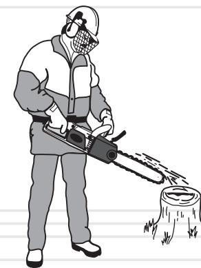
1. Start engine and for 1 minute hold at a height bar nose 15-20 cm above the surface of any light, for example, spread out over a paper sheet or on timber.
