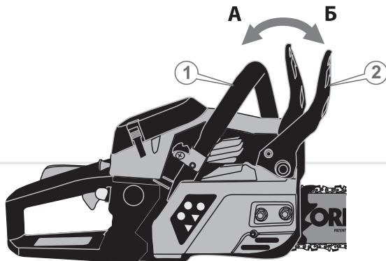
The chain brake is disinhibited (unlocked - chain can rotate) when his arm is in the cocked position (A) - the lever (2) pull towards the front of the handle (1) (see Figure 9).
