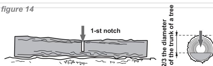
1. Make the first cut down to 2/3 the diameter of the trunk of a tree (see Figure 14).
