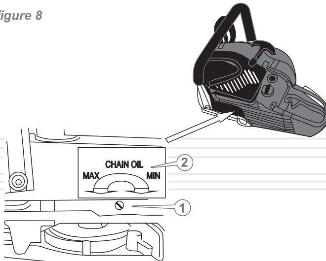
1. Insert a screwdriver into the slot of the stem (1) oil pump.
