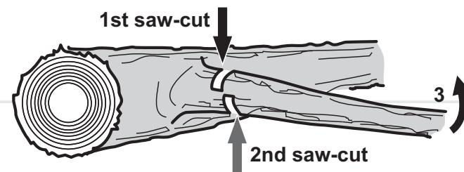
The process of pruning twigs and branches from a fallen tree is very similar to the process of bucking.
