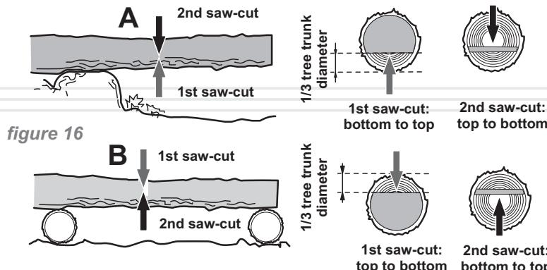
1. Make cuts logs in the "A". Make the first cut from the bottom up (1) 1/3 of the log and finish the cut from the top down.
