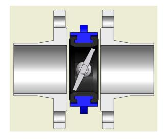
Leave enough space between the flanges so that valve can be easily inserted or removed
