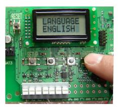
One of the big changes with regard to the previous generation is that from now on all the communication with the CB occurs with an LCD clear display and a 4 knob keyboard. The communication is thus much clearer, and especially since the LCD screen communicates in the language of your choice (F, NL, GB, D).
