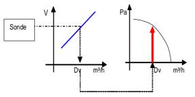
Link between 0/10V signal and constant airflow
