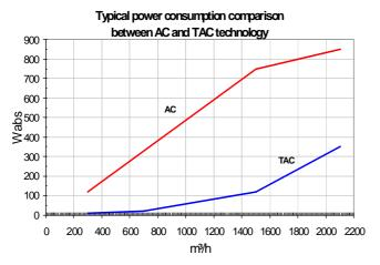
On top of the direct energy saving, there is an indirect one: less electrical consumption means less heat loss and thus in certain cases less cooling load. Less cooling load could mean air conditioning savings, in power consumption and also in investment (smaller units).
