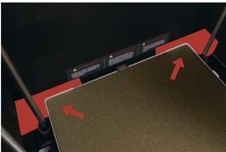
Remove the foam between the hot bed and the inner wall.
