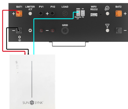
Inverter Unit: 1 External Battery Number: 1
