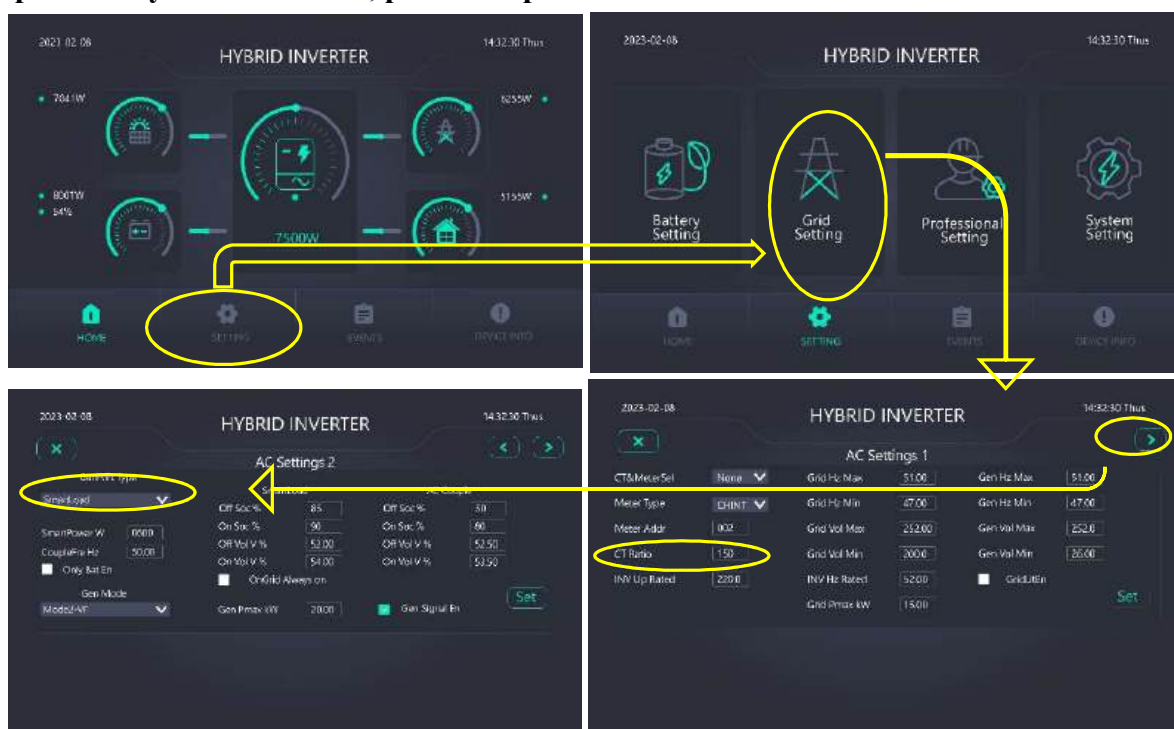
Figure 3.17 Intelligent Load and CT Ratio Setting Path
