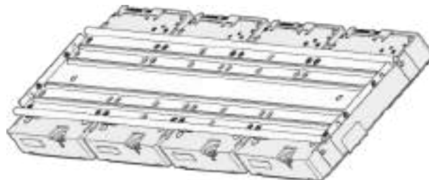
Figure 2-20 Install other HDDs
