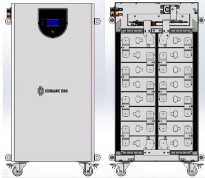
Fig. 3-1 MOON16-G Pro PACK mechanical structure 1
