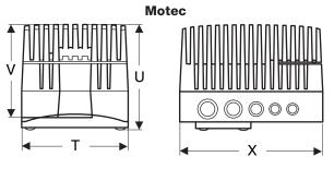
Motec: Direct coupled frequency drive system, integral with the AC motor. Fully variable speed control using a small handheld control pad.
