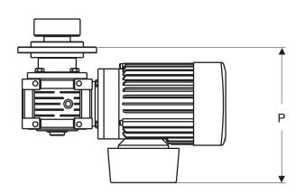
The Motec frequency drive is attached to the AC-motor in 1 of 3 possible positions – please contact Roplan for details.
