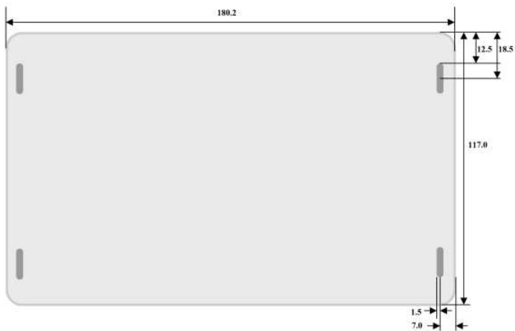
Fig.2-1 Mainboard installation dimension drawing
