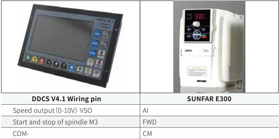
Figure 2-9 DDCS and VFD wiring
