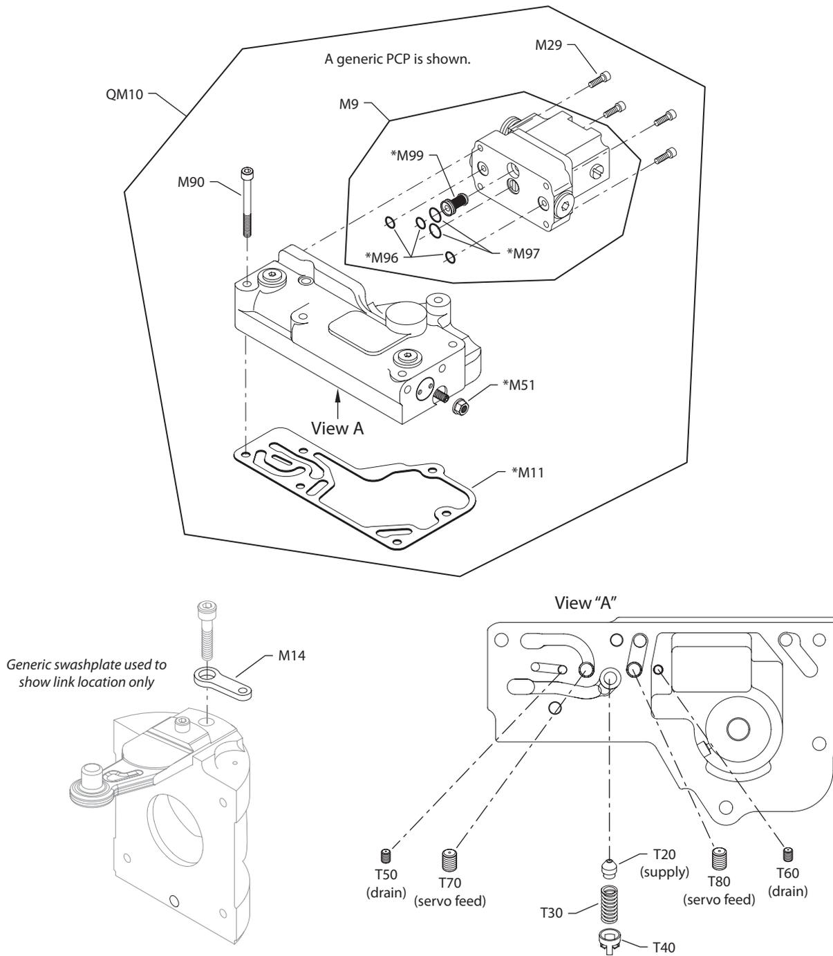
NOTE: All orifices present in the original control must be transferred to the replacement control. If replacement control contains pre-installed orifices, remove and discard them before transferring existing orifices to new control.
