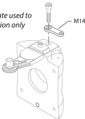
NOTE: All orifices present in the original control must be transferred to the replacement control. If replacement control contains pre-installed orifices, remove and discard them before transferring existing orifices to new control.
