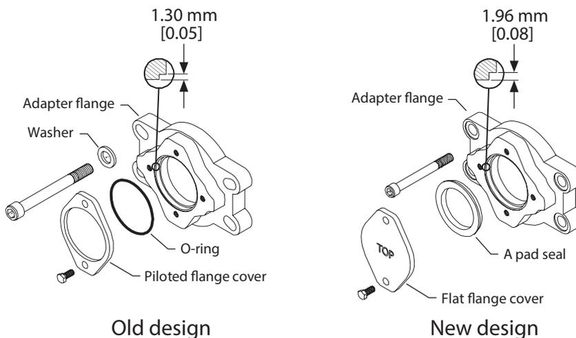
**Models affected** All series 90 42, 130, 180 and 250cc pumps with an SAE A auxiliary mounting flange.
