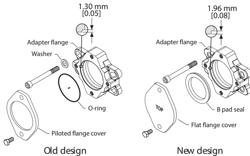
**Models affected** All series 90 42, 130, 180 and 250cc pumps with an SAE B auxiliary mounting flange.
