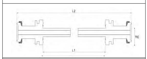
Dimensions for Connectors pump segments (further dimensions on request):
