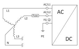
Using a fuse or a circuit break to protect the AC/L2 input is suggested. The AC/L2 input is internally non-protected. Suggested fuse is shown as below.
