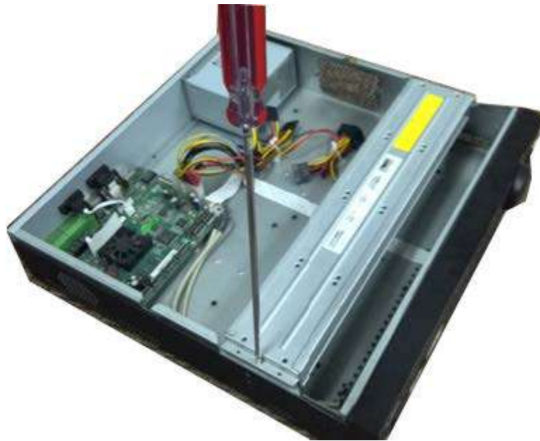
Figure 3-37 Open the top cover
