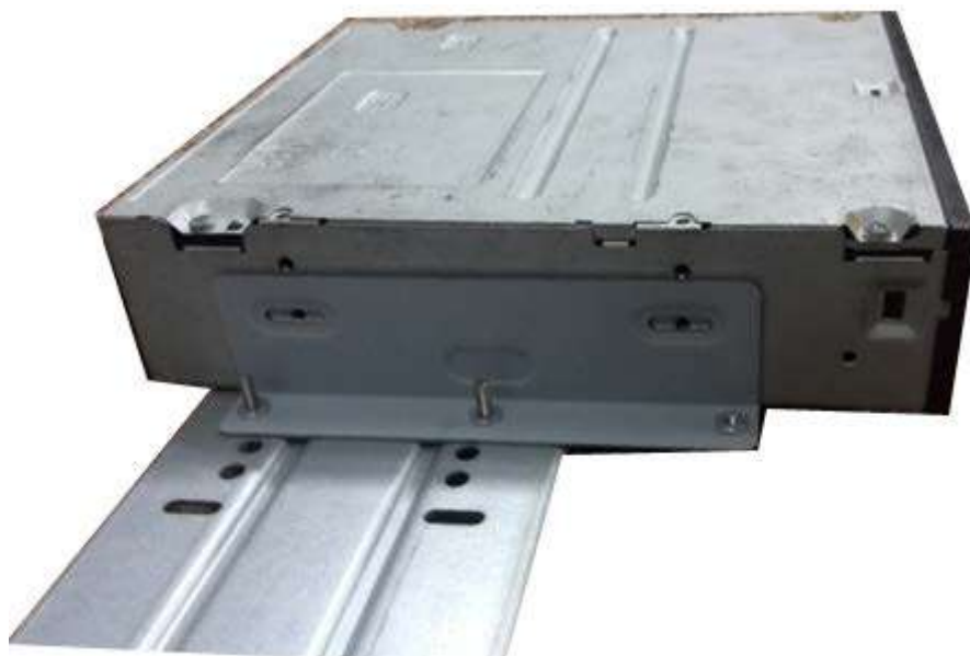
Figure 3-43 Install SATA burner
