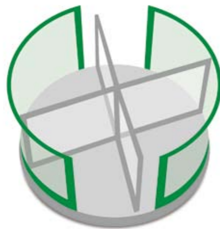
↑ KBB drum wall load-bearing
